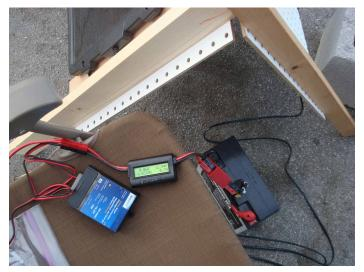
Solar charger controller, meter, battery (early morning so not much current)
