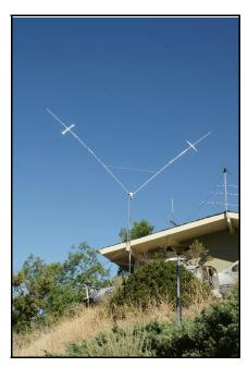
of one in the air and using a slip of paper held against my computer monitor I was able to mark the length of the outboard trap on a piece of paper. Using this as a ruler, I was able to measure the distance to the capacity hats and the length of the adjustable end pieces. The capacity hats were one trap length away and the end pieces were two and a half trap lengths long. Transferring this to the actual antenna was the last step in the assembly.
